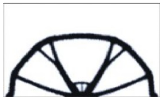
Optimized solid distribution of a bridge by Agyekum [7]
