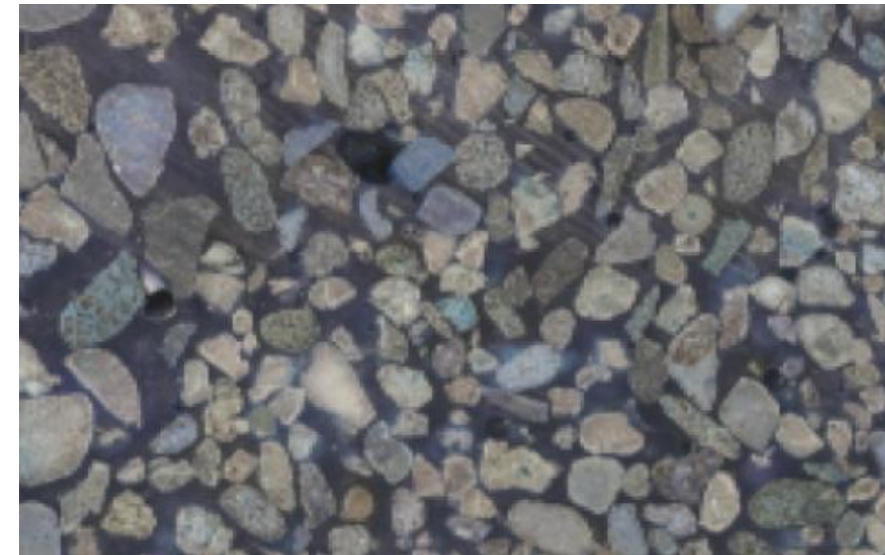
Fig. The slice of the intact clastic rock sample filled with synthetic resin (the photo of cross-sectional plane).
