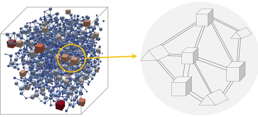
$\diamond$  Thermodynamic equilibrium inside a single pore  $f^{1,k}(p^1, T, x^k) = f^{g,k}(p^g, T, y^k) = f^{ad,k}(p^{ad}, T, w^k)$ Gas fugacity Adsorption fugacity Oil fugacity
