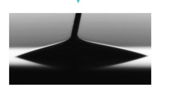
Change in the wetting properties due to an electric field. Experimental images of NaCl solution on silicon.
