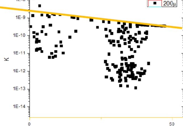
The Darcy's Law give the permeability of the synthetic rocs and the metallic foams by experimental measures using a high pressure chamber. Q= flux, A= area, L=lenght  $\mu$ = viscocity,
